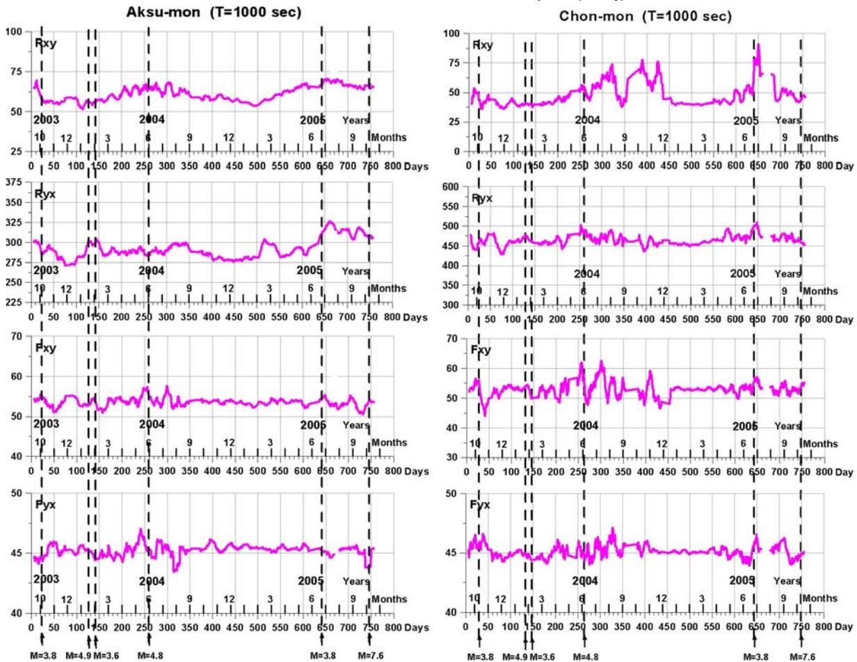
Fig. 8. Resistivity and phase at different periods based on the continuous monitoring of the MT fields. Site Aksu (left panel), site Chon (right panel)
