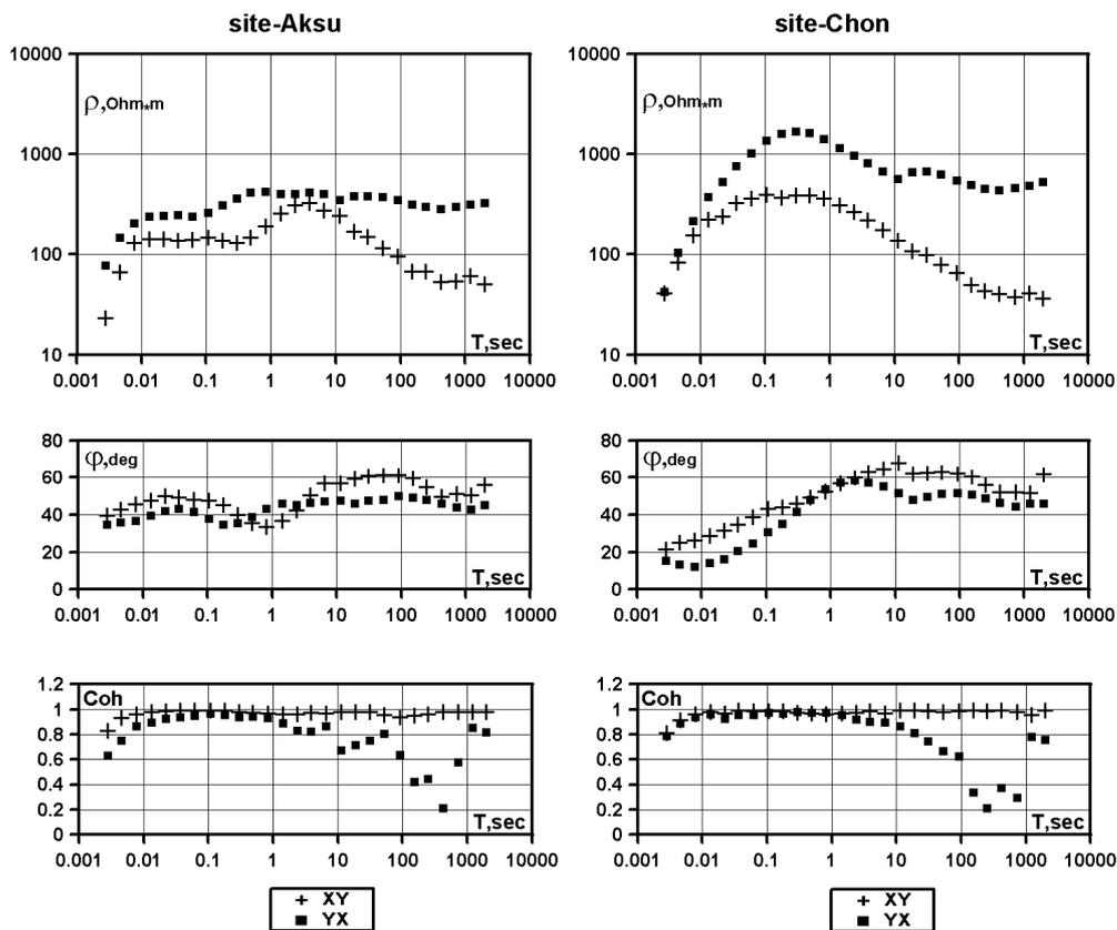
Fig. 4. Reference MT curves (amplitude and phase) and local coherences for monitoring sites were calculated as the median of the 740 daily estimates for two monitoring sites (xy: north-south; yx: east-west)
