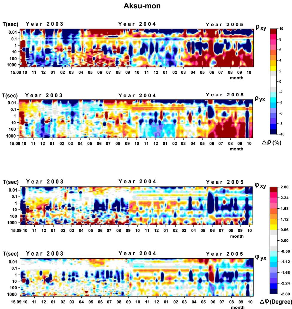
Fig. 5. Frequency-time diagrams of apparent resistivity and phase daily average values obtained at site Aksu. Dynamics of time series is presented by relative differences (in percent and degree) between current and reference MT curves for full set of sounding periods at the given site during September, 2003 – October, 2005.  $\rho_{xy}$  – direction in north-south;  $\rho_{yx}$  – direction in east-west.
