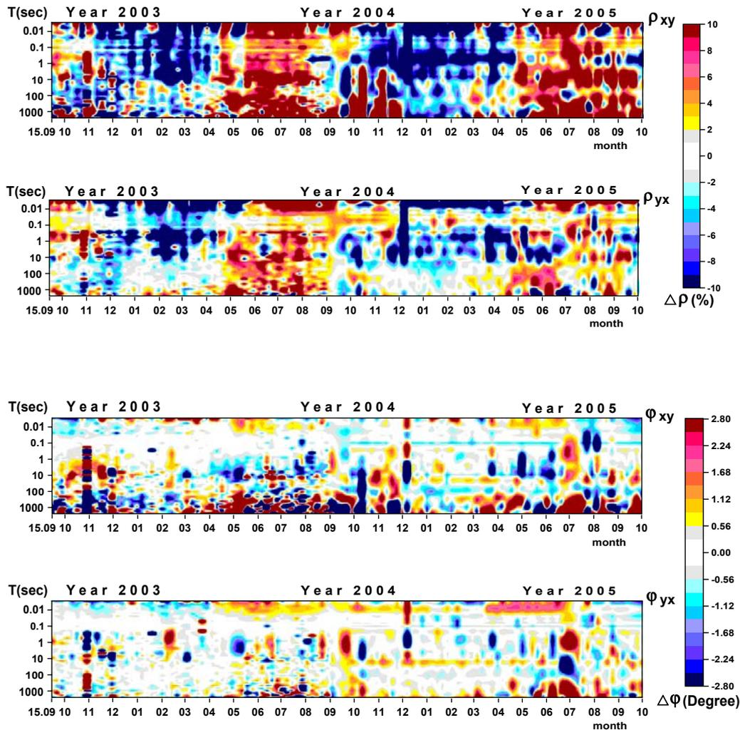
Fig. 6. Frequency-time diagrams of apparent resistivity and phase daily average values obtained at site Chon. Dynamics of time series is presented by relative differences (in percent and degree) between current and reference MT curves for full set of sounding periods at the given site during September, 2003 – October, 2005.  $\rho_{xy}$  – direction in north-south;  $\rho_{yx}$  – direction in east-west.
