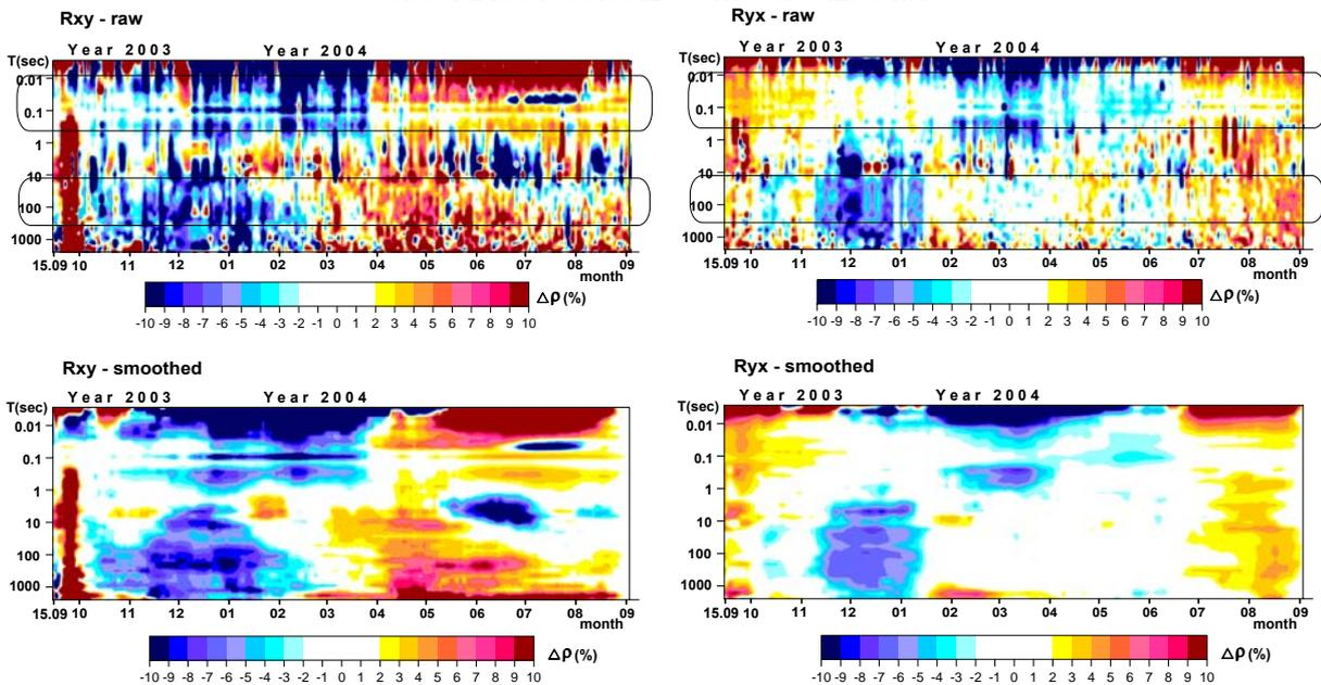
Fig. 7. Raw and low-pass filtered variations of daily averaged estimates of apparent resistivity expressed in percent. The median filter with smoothing window of 11 days was applied in time domain.
