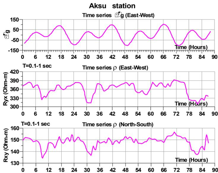
Fig. 3. Comparison of an average apparent resistivity ( $\rho_{xy}$ ,  $\rho_{yx}$ ) in the band 10-1 Hz and calculated gravity variation (in  $\mu\text{Gal}$ ) at the site Aksu. Beginning of comparison – August 12, 2004 at 16-00 of local time.
