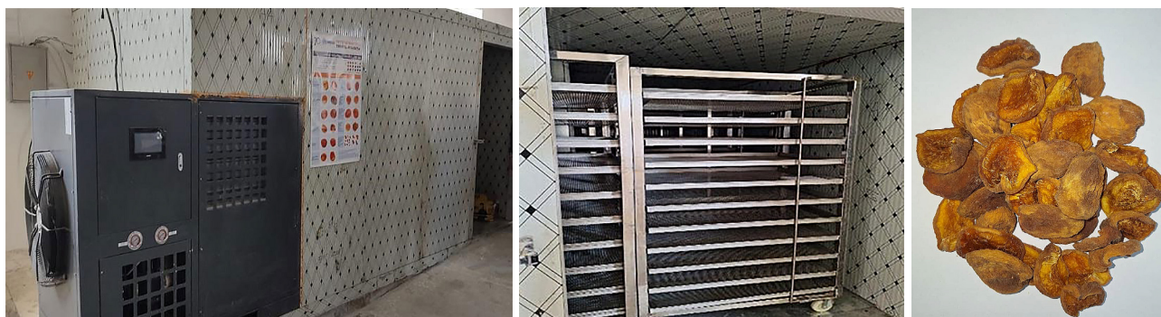
Figure 8. Hot air-dryer used for apricot drying in Batken region, Kyrgyzstan, and dried apricot in hot air-dryer (pre-treated with 1% citric acid solution)
