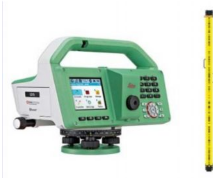
Figure: 4. Leica LS15 digital level and Leica GPCL3 invar staff.
