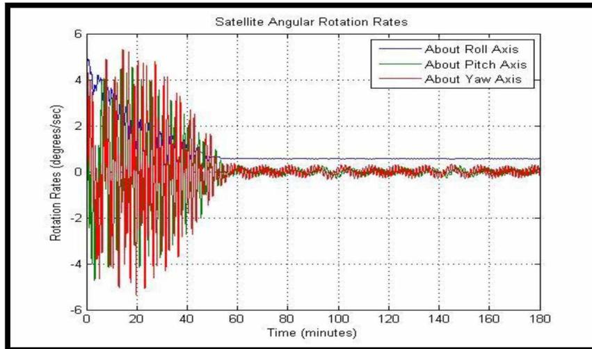
Fig.3 CubeSat angular rotation rates for 2012 mission
