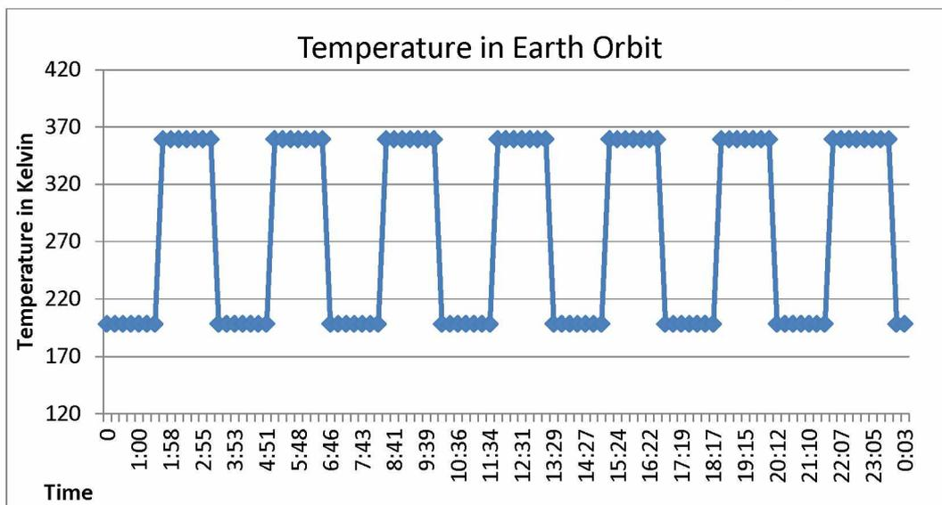
Fig.4 Internal temperature of CubeSat in Earth Orbit for 2012 mission
