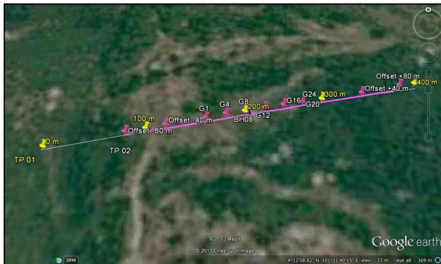
Figure 3: Location of survey lines for 2-D resistivity (yellow) and seismic refraction (pink) (Google Earth, 2010)
