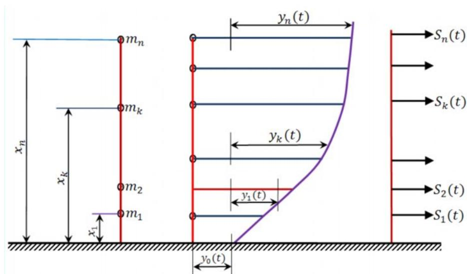
Fig. 1. Calculation scheme of a discrete type
