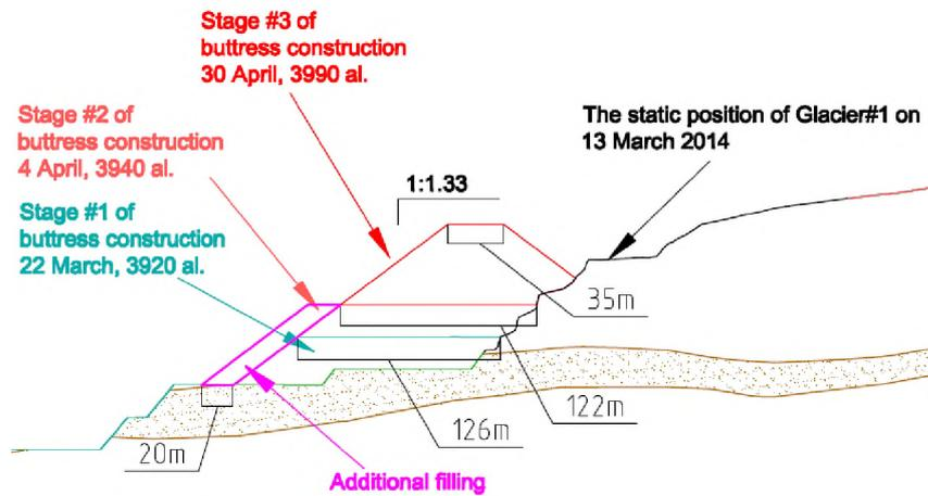
Figure 17. Additional filling in buttress construction.
