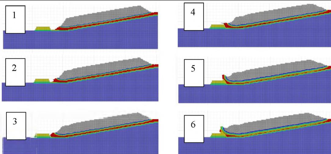
Figure 9. Steps of test model calculation process.
